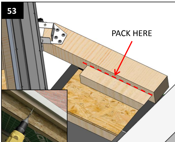
53 Pack if necessary between the timber "A" frame and the panel edging to ensure proper alignment with the exterior panel battens. And centre "A" frame to ridge. Screw up through timber edging as shown inset (see main guide)
