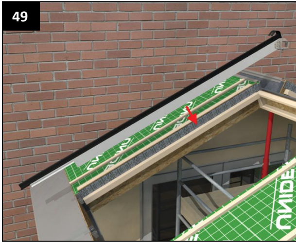
49 Lower the glazing bar into position along the top of the timber panel edging and locate in the eaves beam support shoe (see standard glazing guide)
