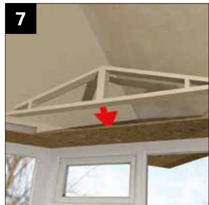
7 Fabricate 70 x 45mm triangular studding framework to suit.
