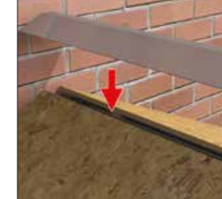
Fixing Aluminium ridge plate
