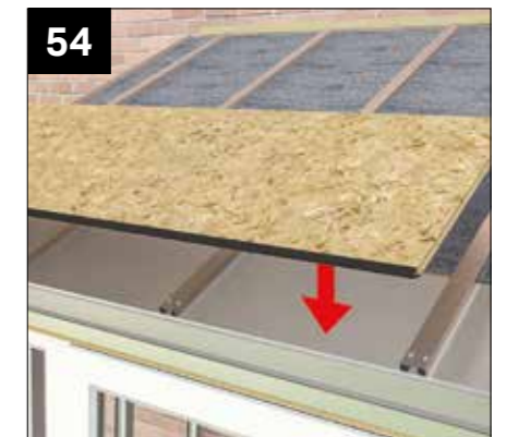
Following location plan, locate first row of OSB panels around the roof using tile starter support section to position. Ensure OSB sheets are the right way up, orientation.
