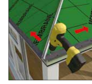
Fixing Ultratile starter strip
