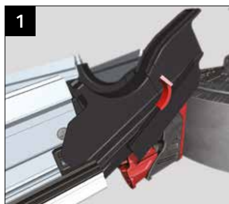
If you need to remove a glazing bar from the speedlok 2 socket assembly, remove the speedlok hood (if fitted) and release and lift the bar at the eaves end.
