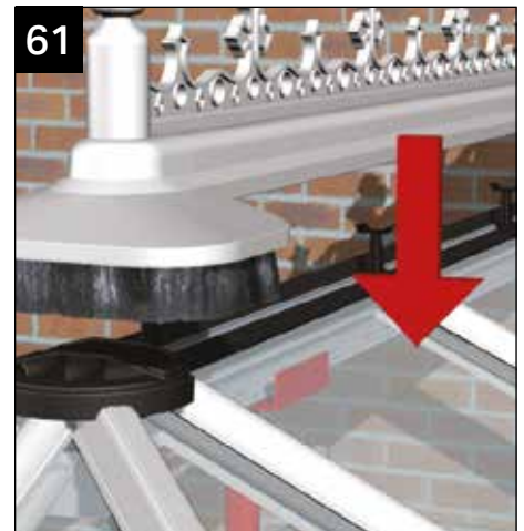
61 Offer up the complete ridge capping onto the roof.
