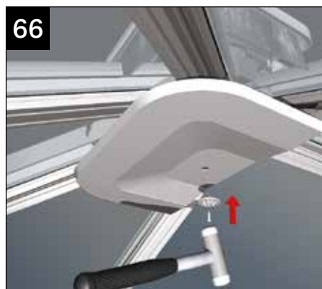
66 To fit the internal radius end capping insert the rose fixing button and tap the plastic rivet home to secure the button. On some occasions it may be preferable to test fit the ridge internal cladding prior to fitting the radius end capping.
