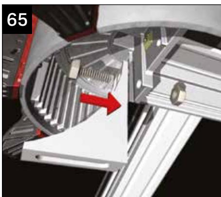
65 Fit the "L" shape PVC bracket to the underside of the radius end. Offer up the internal radius end to check the position of the bracket before tightening.
