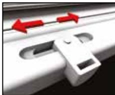
Ensure the ventilation button is fixed into the ridge undercladding as shown before you install the cladding.
