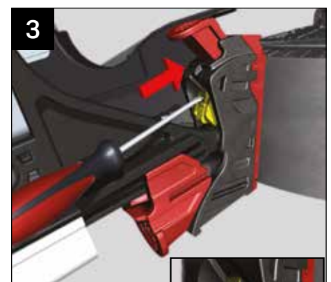
Insert the 5mm wide flat blade screwdriver and gently push against the upper edge of the roller cam (marked yellow).
