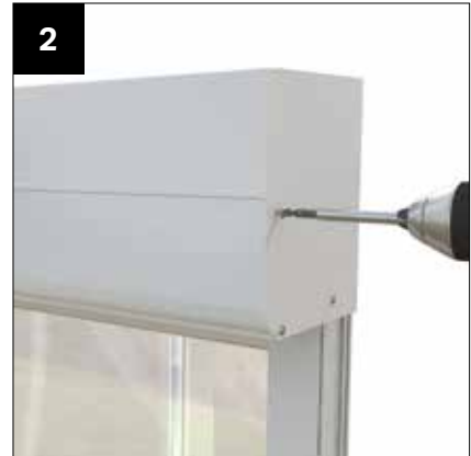
2 GUTTER STOP END DETAIL - Used with lean-to roofs, gable roofs or when then gutter returns along the host wall. Secure the end plate into position using the fixings provided (CRN008).
