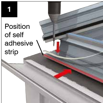
1 Remove under gutter trim, attach self adhesive strip to 'toe' of eaves beam.
