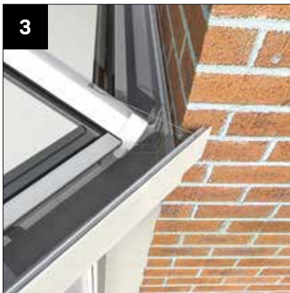
CORNICE BOXGUTTER DETAIL - For situations other than that shown, Cornice should be prepped by you on site to suit the wall condition you find.
