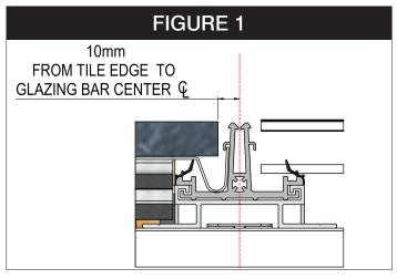
If the roof contains full rectangular glass panels, the starter strips MUST be fitted from the glazing bar.
