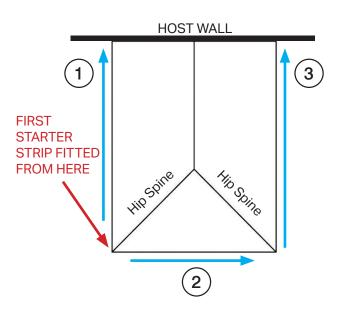
If a roof contains no rectangular glass panels and is classed as 'solid' then starter strips must be set out from the hip spine.
