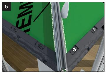
Mark position of hip spines and remove from roof, this helps with fitting of the tile panels.
