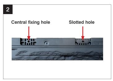
Fix through the central fixing hole for temporary fitting. (DO NOT FIX THROUGH SLOTTED HOLES UNTIL ALL STARTER STRIPS ARE IN PLACE)
