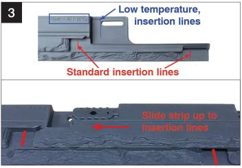
Following the direction stated in the fitting guide (see p1). Align next starter tile strip with the standard insertion lines.
