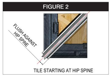
If the roof contains no rectangular glass panels, then the starter strips MUST be fitted at the hip spines first.
