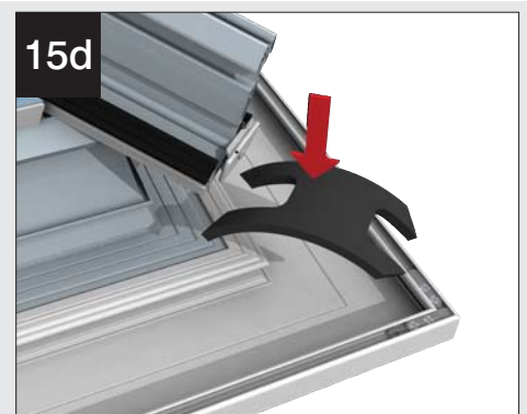
At 90° corner insert 'H' section and press down. Similarly apply at stop end or outlet positions.
