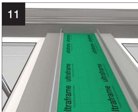
11 Silicone along faces of cladding clips as shown by.
