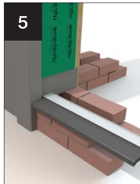
This is the detail you will create on the 130 mm cill.
