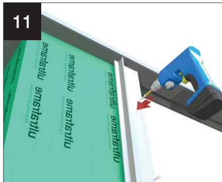
11 Remove black PVCu brick spacer extrusion and then fit cladding clips to columns. Clips are used to position windows
