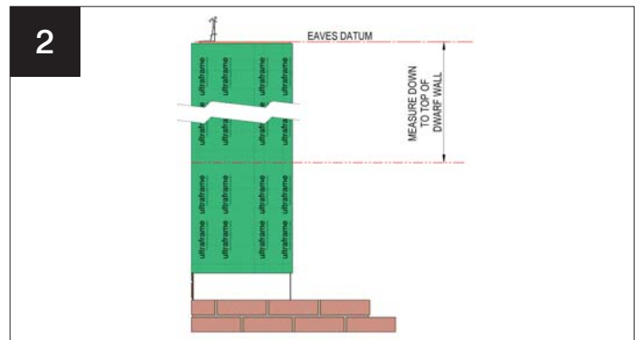
2 If building dwarf walls, measure down from underside of eaves and mark column to set datum for dwarf wall height. This ensures that window opening is correct. FITTERS TIP: FASTEN STRINGLINE BETWEEN COLUMNS
