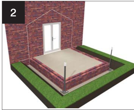
2 Complete base to slab level. Note: If fitting columns directly on cill remove set out posts.
