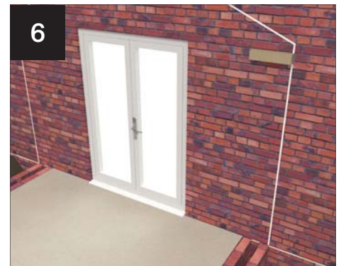
6 If no abutment column specified temp fix timber batten on host wall at eaves level. (Underside of eaves beam)
