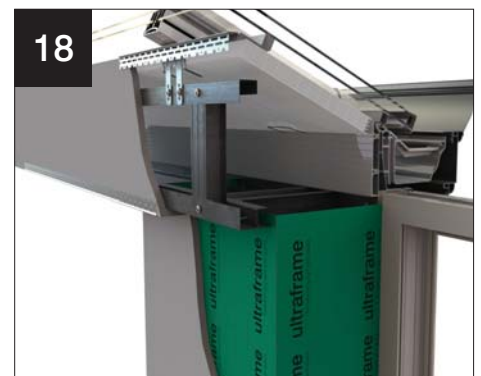
18 Fit insulated internal pelmet (if specified) and plasterboard
