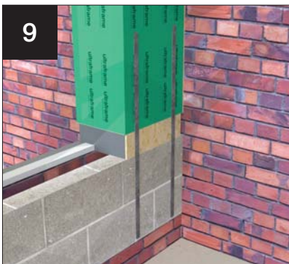
ABUTMENT Fasten straps down inside of wall of abutment column.
