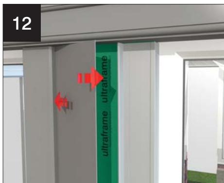
12 Locate infill panel between cladding clips and push against silicone.
