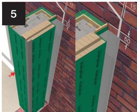
5 Fit abutment column to bracket and temp fix with one screw. Bracket should be 50mm below bottom of eaves beam.
