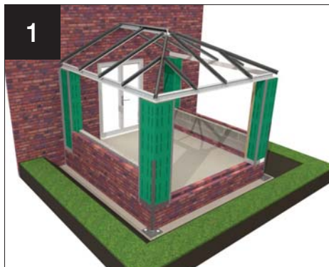
Fit windows between columns.
