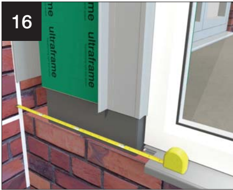
16 If abutment plinths are specified, measure the distance from the cill prep to the house wall.
