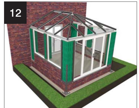
12 Fit and seal windows/doors against clips
