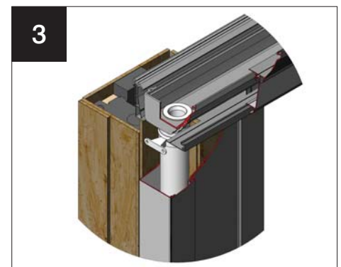
Cornice shown in situ with concealed downpipe.
